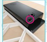
Once assembled, flip the power switch to ON. The switch is located on the battery compartment
