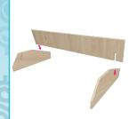
Insert the long, wooden base with the slots facing down into the short side of the support pieces as shown in the image.
